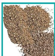
**PERSNICKETY® Media** Converting/Polishing media is impregnated with a patented polymeric amine and is used in high  $H_2S$  conditions. Oxidizing/Polishing media is impregnated with Chlorine Dioxide and is used in low  $H_2S$  conditions. Disposal is not an issue when the media is changed out as recommended by the manufacturer.
